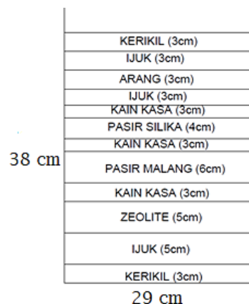
Gambar 2. Susunan Media Filter
