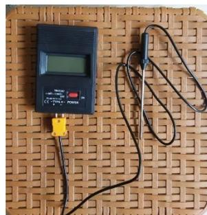
**Gambar 4 K Type Digital Thermometer.**
