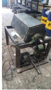
**Gambar 10.** Mesin Barel Polishing
