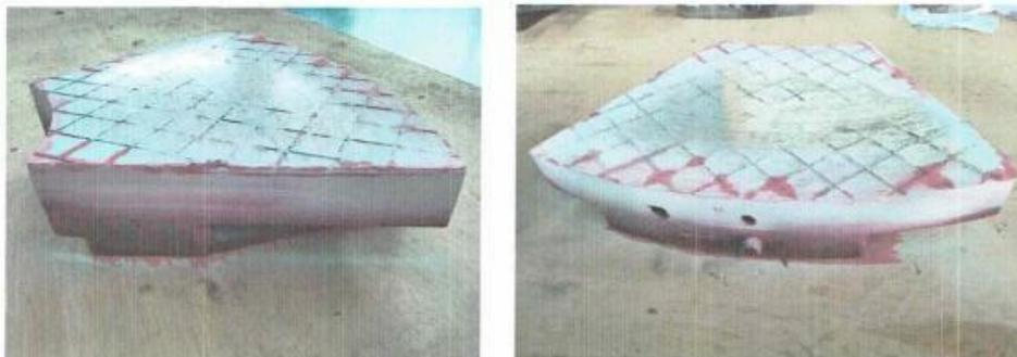
**Gambar 3.** Pad thrust bearing (terkikis)
