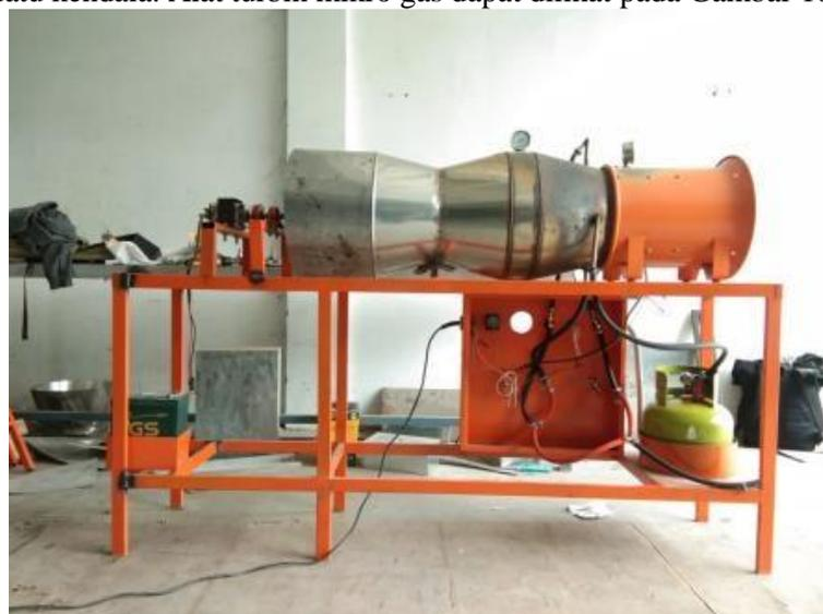
**Gambar 10.** Alat Turbin Gas Mikro.
