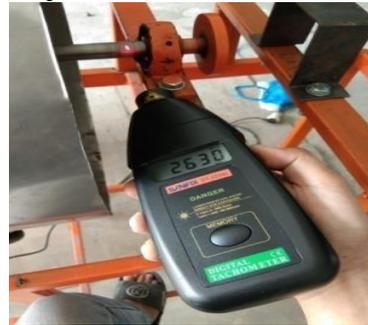
**Gambar 12.** Tachometer digital
