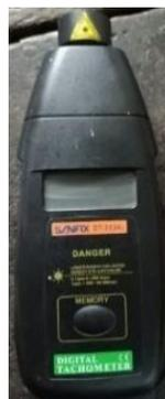
Gambar 3. Alat ukur tachometer
