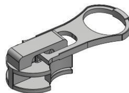
10) Gambar 5. Automatic Lock Slider: Leaf Spring
