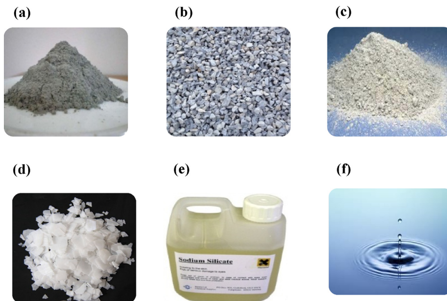
Fig. 1. All the materials used to fabricate the GPB concrete with (a) fly ash, (b) coarse aggregate, (c) fine aggregate, (d) NaOH, (e) \text{Na}_2\text{SiO}_3 , and (f) water.
