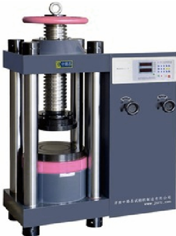
Fig. 2. Compression testing machine used to measure the compressive strength of GPB sample.
