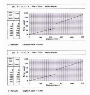
Figure 1 : UPV Test before injection
