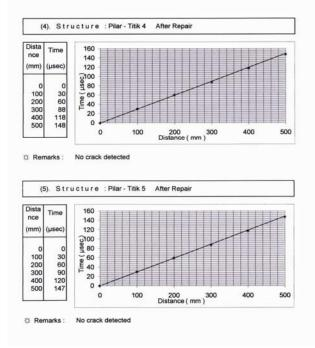
Figure 2 : UPV Test after injection
