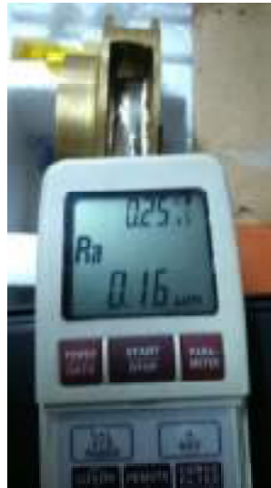
Figure 5. Measurement of surface roughness of the blade impeller
