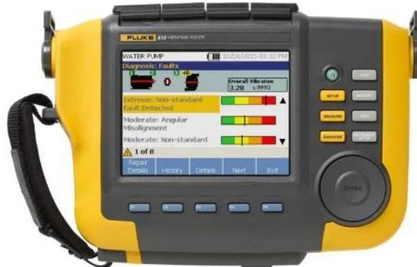
Gambar 4 Alat ukur *vibration tester*
