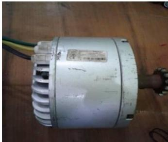
Gambar 2 Brushless direct current motor [7]
