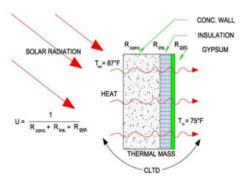
Figure 5: Heat gain through walls with radiation load
