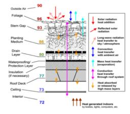
Figure 7: Vegeted roof layer temperatures at afternoon (degrees) oF [14].
