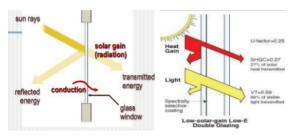
Figure 8: Heat transfer glazing [15]
