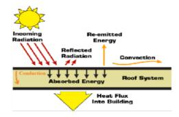
Figure 6: Energy balance on roof surface
