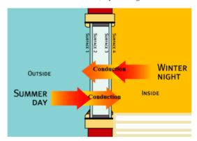
Figure 10: Heat transfer in the door [16]
