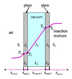
Figure 9: The net heat transfer in glazing
