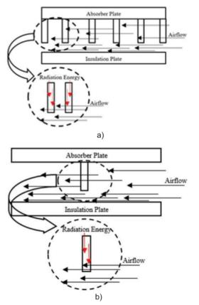
Figure 10: Heat transfer process on multiple fin elements (a) and single fin elements (b)
