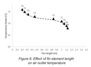
the solar air heater pipeline to decrease. In addition to the outlet air temperature condition, the air temperature conditions in some parts of the solar air heater can be analyzed by the equations calculation among others are air temperature in the collector plate, absorbent plate, top-bottom section pipe duct, and insulation plate, where it can be shown by equation 8 until equation 11. The calculation results can be seen in Table 2.
