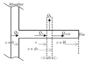
Figure 4: Energy balance scheme of fin elements
