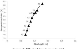
Figure 7: Effect of fin element height on air outlet temperature
