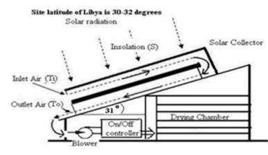
Figure 2: The solar air heater with double-pass type
